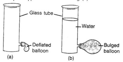
A deflated balloon is tide on the side tube of container opened at one side. Now fill water in the container, balloon connected inflats due to pressure of liquid exerted side ways. This shows that liquids exerts pressure sideways also.
