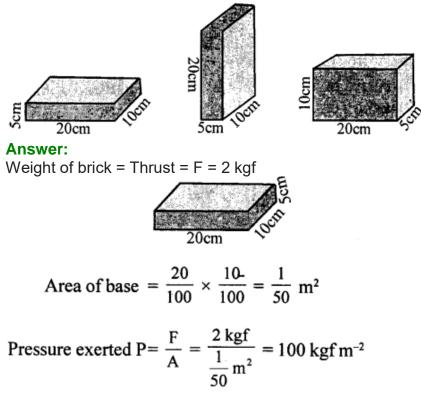
Or Area of base = area of top L × B 20 Cm × 10 = 200 cm<sup>2</sup>  $\mathbf{P} = \frac{\text{Thrust}}{A} = \frac{2 \text{ kgf}}{200 \text{ cm}^2} = \frac{1}{100} = 0.01 \text{ kgf cm}^{-2}$ (b)
