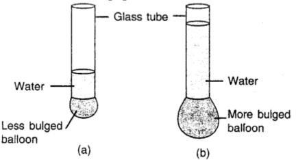
(a). Now add more of water in the tube bulging also increases. Add still more water bulging also increases further as liquid pressure at a point increases with increase in height of the liquid column above that point.
