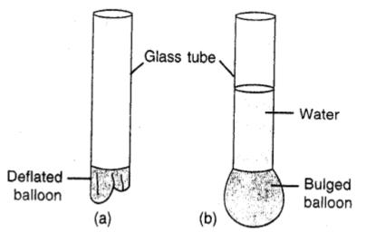
Take a balloon and tie it at the lower end of a glass tube and hold vertically as in fig. (a) pour some water in the tube, balloon bulges out as in
