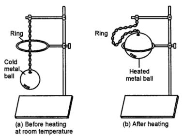
Take metallic ball and ring so that ball can pass through ring easily. Now heat the ball. We see that heated ball cannot pass through the same ring. This is because on heating the ball increases in size. Now on cooling the ball again it can pass through the ring. This experiment shows that solids expand on heating and contract on cooling.
