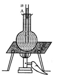
OR Experiment :Take a laboratory Celsius thermometer Suspend it with the help of a stand. Note the level of mercury thread in it. Let it be at A. Now take hot water in a beaker and as shown, set up the arrangement. The mercury thread rises to B by gaining temperature.
