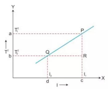
From this graph, the value of acceleration due to gravity (g) can be calculated as follows. The slope of the straight line can be found by taking two points P and Q on the straight line and drawing normals from these points on the X- and Y-axis, respectively. Then, the value of T2 is to be noted at a and b, the value of I at c and d. Then,
