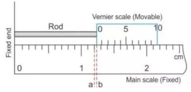
In this position, the zero mark of the vernier scale is ahead of 1.2 cm mark on main scale. Thus the actual length of the rod is 1.2 cm plus the length ab (i.e., the length between the 1.2 cm mark on the main scale and 0 mark on vernier scale).
