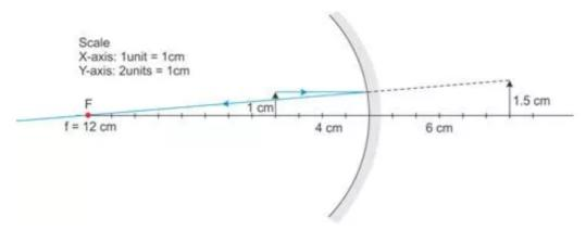
A ray passing parallel to the principal axis passes through the focal point after reflection. Hence, the focal length is 12 cm.
