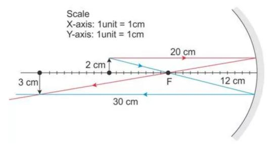
The image is 30 cm in front of the mirror, 3 cm high, real, inverted and magnified.
