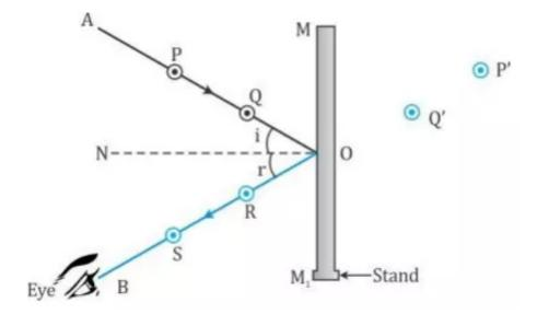
Next fix two pins P and Q at some distance ( $\approx 5$  cm) apart vertically on line OA, on the board. Keeping eye on the other side of normal (but on the same side of mirror), see clearly images P' and Q' of the pins P and Q. Next fix a pin R such that it is in line with the images of pins P and Q as observed in the mirror. Next, fix one more pin S such that the pin S is in line with the pin R as well as images P' and Q' of pins P and Q.
