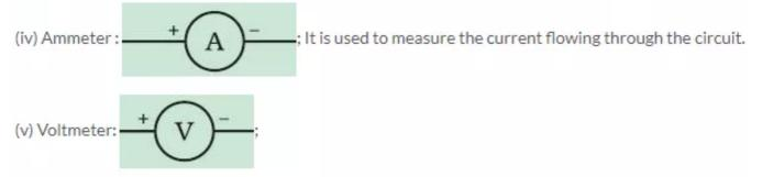
It is used to measure the potential difference between two points of a circuit.
