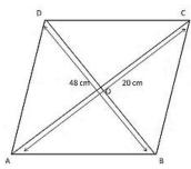
ABCD is the rhombus and AC and BD are the diagonals. The diagonals intersect at point O.
