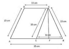
Trapezium ABCD is divide into parallelogram AECD and triangle CEB.
